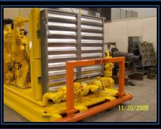
SKID: HEAVY DUTY 4 RUNNER WITH BUMP GUARDS, DESIGNED FOR WINCH TRUCK WITH TAIL ROLL
