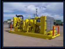
ENGINE: CATERPILLAR INDUSTRIAL DIESEL C18 TIER 3 MAX. HP 630 MAX RPM: 2100
